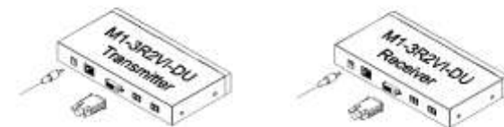
Figure 8 – Connection of AC/DC power adaptor
